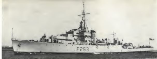
HMS Helmsdale continued to serve for some years after the war as an A/S Trials Ship. She had no gun-armament, but carried twin Squid Mortars on her forward 4 inch gundeck, and retained the D/C arrangements aft.
